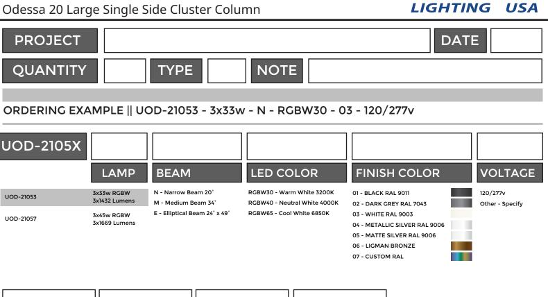
**ADDITIONAL OPTIONS** DIM - 0-10v Dimming A51814 - Linear Spread Lens A65091 - STICK-KE2 A64791 - RDM DMX Splitter NAT - Natatorium Rated A54531 - Anti Glare Louvre A68391 - STICK-DE3 A65191 - TPC Touch Panel A54431 - Anti Glare Visor A54121 - Honeycomb Louvre A64491 - TPC + DMX Controller A65391 - EDN Ethernet Data Node A64591 - POE Connect A66991 - LPCX Lighting Playback A64691 - TPC + DMX 2 A64991 - CLOUD
